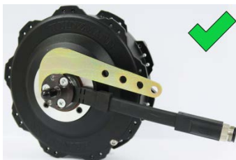
Right, with torque support and stub axle
